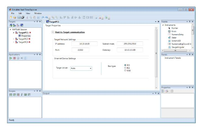
**Note:** In R2017a, support for using ISA bus Ethernet cards to communicate between the development and target computers will cease to function. Use PCI bus or USB bus Ethernet cards instead.
