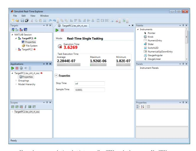
If you choose a sample time that is too small, a CPU overload can occur. If a CPU overload occurs, the target object property CPUOverload changes to detected. In that case, change **Fixed step size** to a larger value and rebuild the model.
